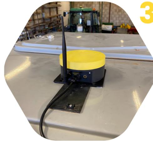
**3** Install FieldBee controller on the tractor's roof
