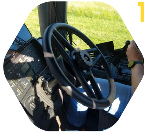
**1** Replace steering wheel with PowerWheel
